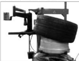
Demounting lower bead
